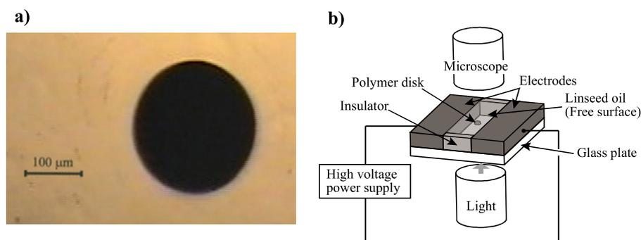
**Figure 2.** Top view of a gelatine based composite (a), and the experimental device used to study the Quincke rotation (b).
