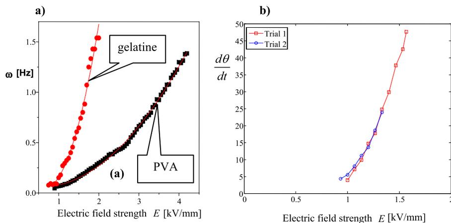
**Figure 5.** Dependence of the rotation frequency (a) and angular frequency (b) as a function of the DC electric field. (a) Disk diameter:  $240 \mu\text{m}$ , disk height:  $80 \mu\text{m}$ ; FeO(OH)/gelatine mass ratio: 2.67. (b) Disk diameter:  $573 \mu\text{m}$ , disk height:  $208 \mu\text{m}$ ; FeO(OH)/PVA mass ratio: 8.4.
