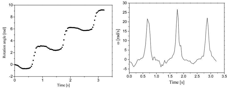
**Figure 6.** Dependence of the rotation angle (a) and speed of rotation (b) on the time at  $E = 1.33 \text{ kV mm}^{-1}$  AC field intensity with  $f = 0.9 \text{ Hz}$ .
