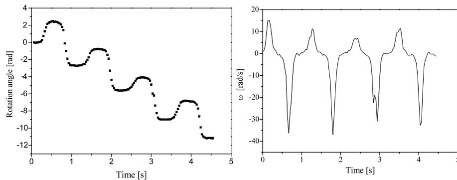
**Figure 7.** Dependence of the rotation angle (a) and speed of rotation (b) on the time at  $E = 1.5 \text{ kV mm}^{-1}$  AC field intensity with  $f = 0.9 \text{ Hz}$ .
