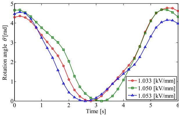
**Figure 4.** Dependence of the angle of revolution on the time slightly above the critical threshold. The applied electric field intensity is given in the box.
