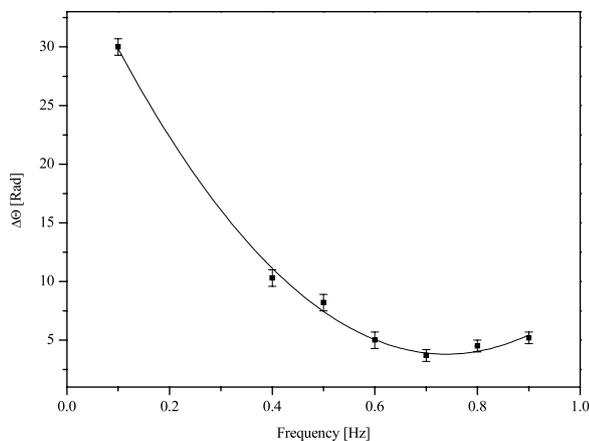
**Figure 8.** Dependence of the maximum angular displacement on the frequency measured at  $E = 1.5 \text{ kV mm}^{-1}$  AC field intensity. The solid curve is a guide for the eyes.
