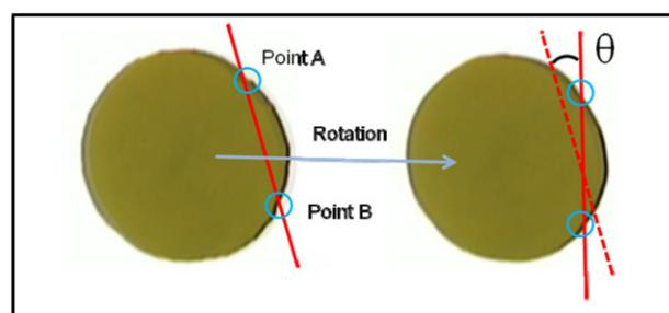
**Figure 3.** Determination of the angular displacement. The angle between the dotted and straight lines characterizes the angular displacement.
